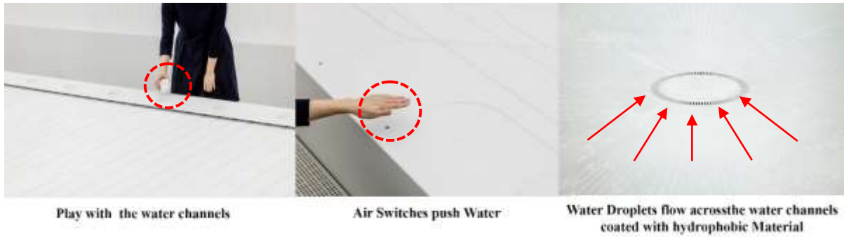
Fig. 4. Ergonomic air switches push water into the channels when a visitor hovers his or her hand over the air holes.
